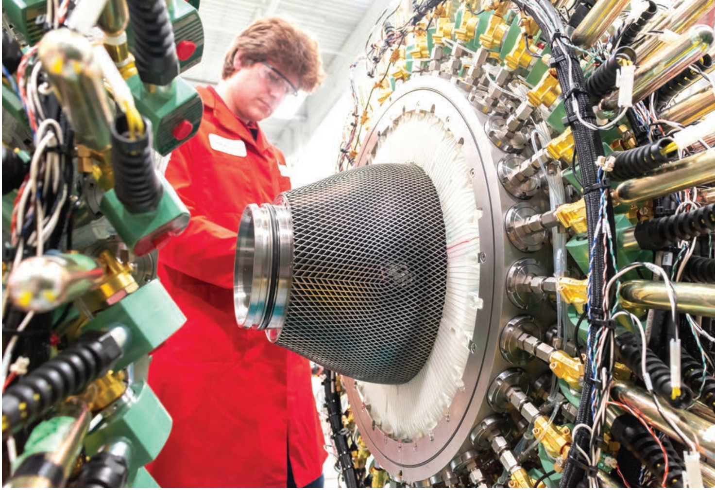
3D titanium parts being installed in compression test chamber (image by Tim Howard/General Fusion)
